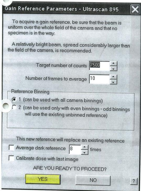
If specimen/rod is inserted for capture the night before, pull out rod to the first hold position (pull out until it stops and turn counter clockwise until resistance is met). Turn on beam (1 and 1/2 minutes), center it, and spread a couple of partial turns outside the edge of the screen. All values in adjacent window are default. Click YES to proceed.
